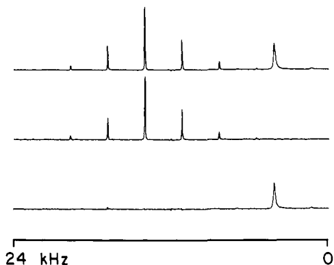
Figure 7. Glycine spectra from Figure 6 for t_1 = 0 (top) and t_1 = 100 \mu\text{s} (middle) and their weighted difference (bottom). The centerband and sidebands on the left are due to the -\text{CO}_2^- while those on the right arise from the -\text{CH}_2^- . Note the clean separation of the resonances due to protonated and nonprotonated ^{13}\text{C} 's.
